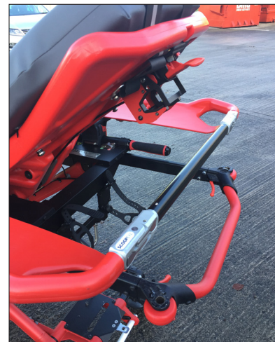
Re-connect Scoop at head- end with a TSL extension pole
