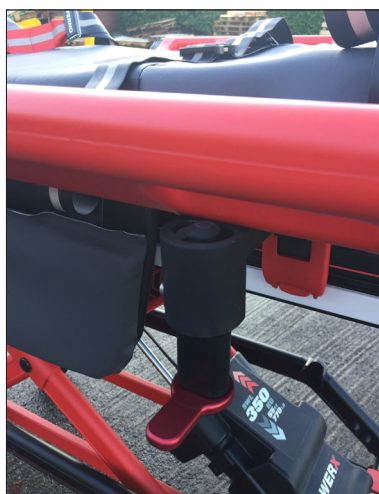
Locking arm unlocked
