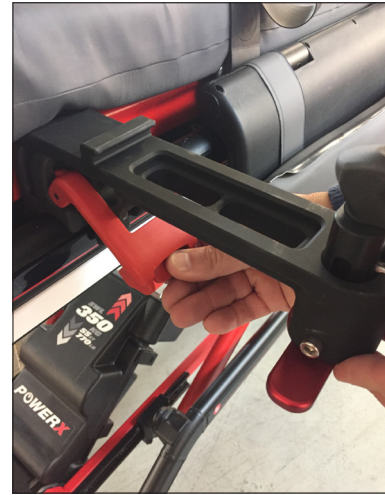
Lock the bracket in place by pressing down on the red locking handle
