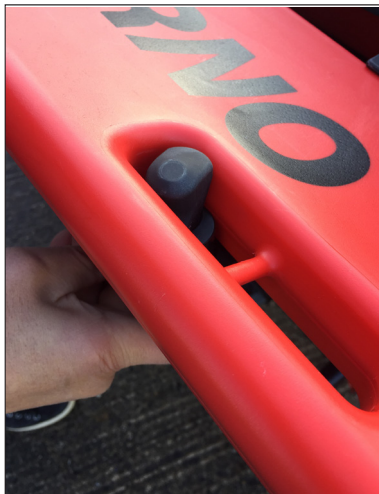
Ensure Scoop hand-hold holes line up with locking arms on fixing brackets
