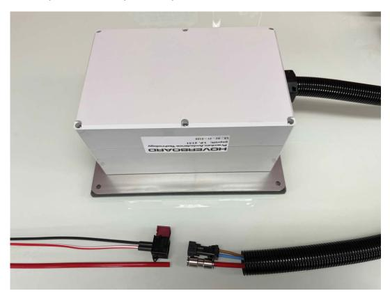
Fasten the box in a suitable place underneath the vehicle, preferably in the rear area, but by never close to the exhaust or in an inaccessible place that causes difficult replacement of the compressor!
