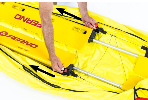
Figure 4 – Rescue bag length adjustment
