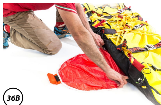
Figure 36 – Placing the sail in the pocket
