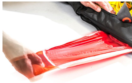
Figure 35 – Taking out the EARS anti rotation sail
